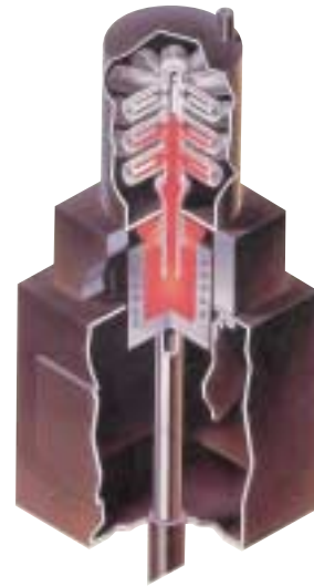
CLV process ( Counter Gravity Low- Pressure Vacuum Casting )
